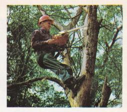
TREE SURGEONS AND UTILITY CREWS like the ease with which they can take the XL-660 Automatic right up into the trees for tree maintenance work. Gear driven, positive-displacement automatic chain oiler eliminates manual chain oiling, greatly prolongs bar and chain life.
