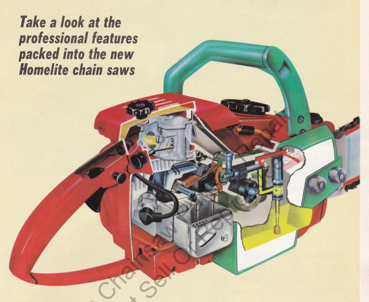
Famous Homelite Short-Stroke Engine—has more powerper-pound. Short piston stroke cuts friction, increases engine life, reduces gas consumption.
