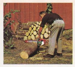
FARMERS make extra cash with the XL-Automatic, because even a few hours cutting on the wood pile turns trees into money. XL-Automatic makes cutting simpler and easier with such features as the automatic clutch which prevents engine stalling if chain binds in cut.
