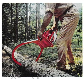
Production cutters in the South have a choice of standard bar, clearing guide or bow.
