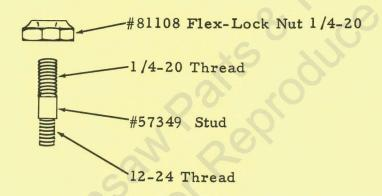
Stud #57349 may be used together with nut #81108 to replace the  $12-24 \times 5/8$ " filister head screw used previously to secure the tank. The clearance hole in the ear of the tank should be enlarged to 17/64" to allow the tank to fit over the new stud.
