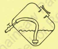
Now it's an interesting fact that we can't get fuel out of the tank, unless we let air in. It works just like your picnic cooler -- you have to loosen the cap before it pours well. In our fuel tanks we have the added problem that we don't want to spill any fuel when the engine is turned upside down. We accomplish this "venting" as it is called through our fuel cap valve.
