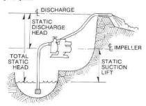
Static Discharge Head — The vertical distance from the center line of the impeller on the pump to the point of discharge or liquid level when discharging into a tank where the pipe is immersed in the liquid.
