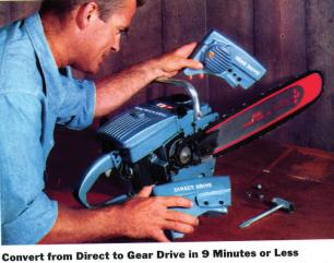
Just remove two nuts and the clutch drum, attach Homelite's planetar conversion unit, tighten it up and you're ready to begin cutting with
