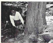
ENGINE TYPE — HOMELITE two cycle, loop scavenged single cylinder
