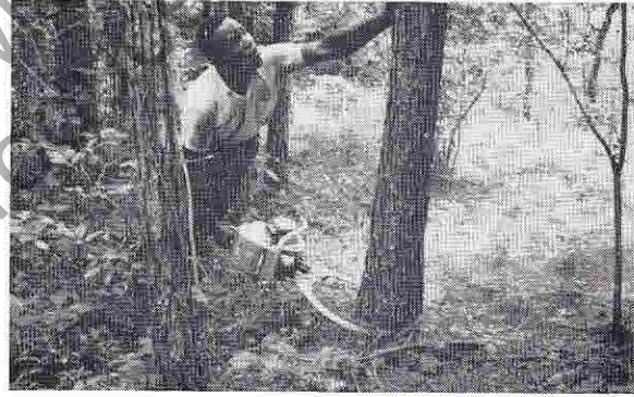
A Super Wiz 66 with bow attachment is used to fell this small tree which the operator can actually then push over with his hand.
