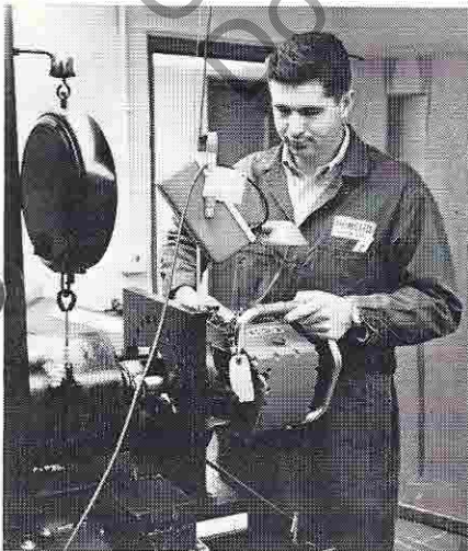
Jerry Karczmit, Development Technician, mounts a chain saw for cooling and air delivery tests.
