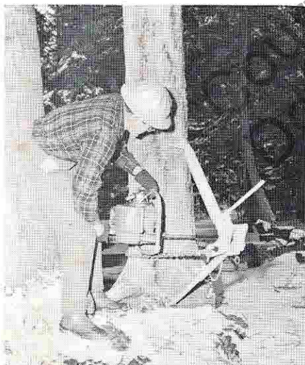
The lower leg of the Directional Tree Faller is placed against the tree at ground level and held tight with a chain. The upper leg or hydraulic ram assembly then slides into the base plate. A loose adjustable sleeve with prongs is slipped over the ram. The operator has made his "overcut."
