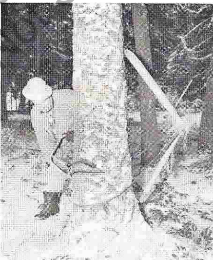
The inventor of the Directional Tree Faller, Arthur Trott, makes the final cut which must be \frac{1}{2} " below the "overcut" on the opposite side of the tree to prevent the possibility of sliding the trunk off the stump. The equipment provides power and safety of operation.
