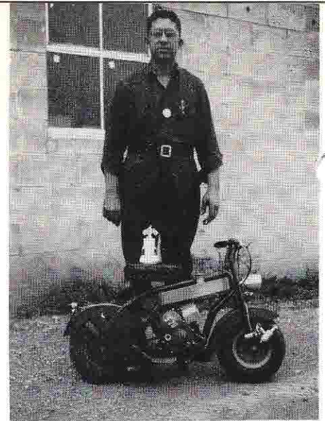
Anthony Arnold of Marietta, Ohio, and the scooter he built around a 5-20 chain saw engine.
