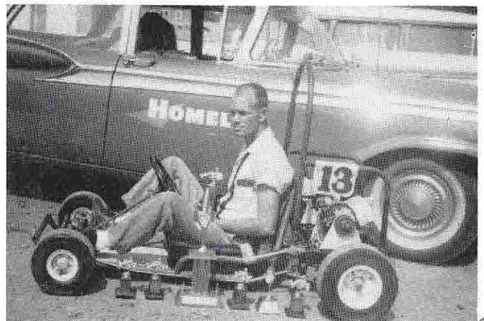
Jim Hoover, above, of Hoover Wheel Sales, Akron, Ohio, poses with his Spitfire, powered by 2 K-92 engines and a few of his trophies. He broke the track record, racing a "B" kart in a "C" race, by doing 1/8 mile in 11.77 seconds. Don Brancaccio, Cleveland Salesman, sent in the picture and information. Jim is holding the trophy he won for his record performance.
