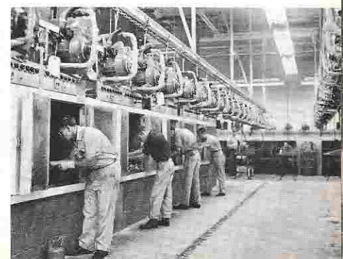
The Test Room has sound proof booths in which each unit is individually tested before final acceptance.
