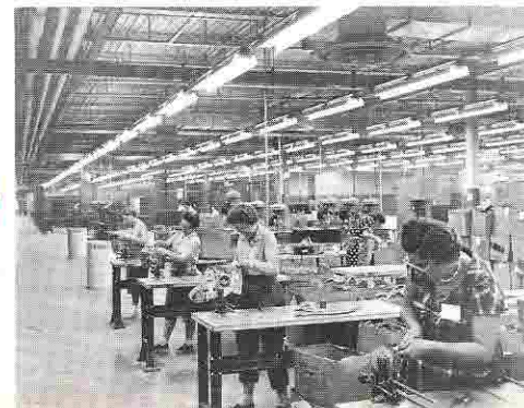
Getting the machined parts ready for the Finishing Department, these women file and smooth the rough edges.
