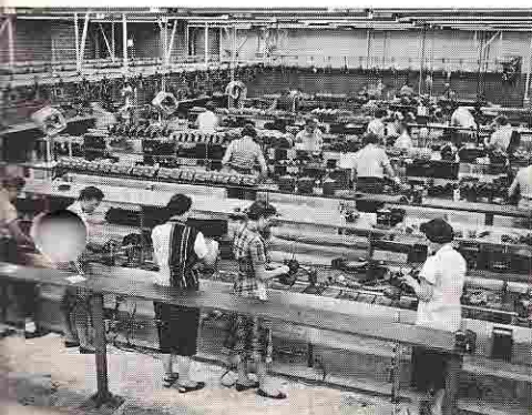
A section of the huge Assembly Department, showing assemblers working on units, moving past on conveyors.
