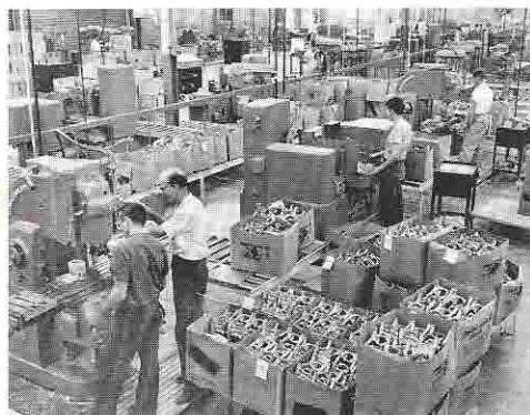
Section of the machine shop with two of the new Cincinnati milling machines and a Heald Boro-matic.
