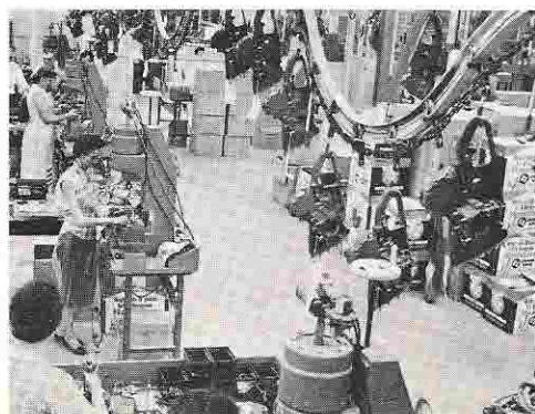
The overhead conveyor dips down at several places for easier, safer handling of the nearly-assembled units.
