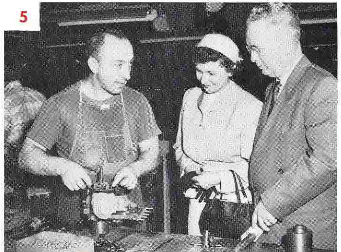
Steve Olszewski explains to the Willsons how he combines five previously assembled parts to make the magneto which he joins to the crankcase. A well planned, steady supply of these sub-assemblies (the responsibility of the Production Control Department) makes this final assembly move quickly and efficiently. Another example of Homelite's fine teamwork.
