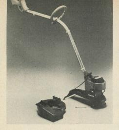
The best new idea in lawn cleanup this year may be this snap-on blower attachment introduced by the Homelite Division of Textron Inc., for its gasoline-powered ST 100 string trimmer. The unique accessory weighs only four ounces and can be attached to the trimmer's power head in seconds. And no tools are required.
