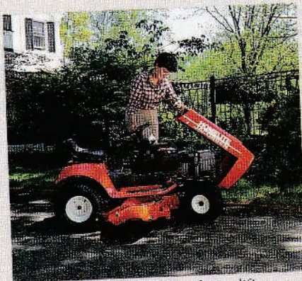
The LTX's easy-to-open hood simplifies maintenance
