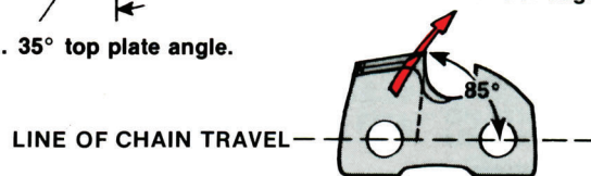
3. Side plate 85° to line of chain travel.
