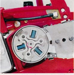
NEW STRONG CLUTCH. Designed to absorb greater shocks and stress. 3 Heavy shoes provide smooth engagement. "Fully floating" needle roller caged bearing with cadmium plating gives longer life.
