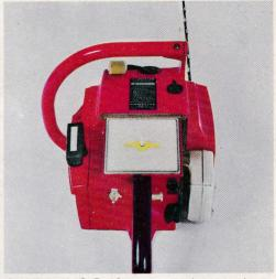
**SIMPLE TO SERVICE.** Takes only seconds to change felt fuel filter. Remarkable Micro Mesh Fibre air filter can be brushed clean or washed in straight Petrol.
