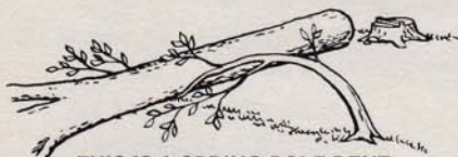
THIS IS A SPRING POLE BENT DOWN UNDER HIGH STRESS.
