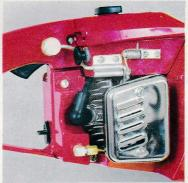
NEW EASIER STARTING. New compression release reduces operator starting effort. New compression release reduces wear on starter. Automatically actuated by throttle lock makes operation
