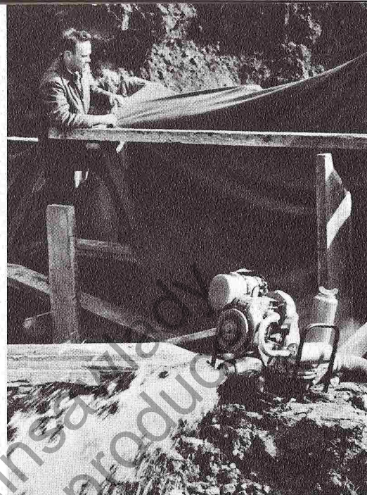
Contractors often have to pump water that's thick with mud or sand. This Homelite diaphragm pump will do the job easily.
