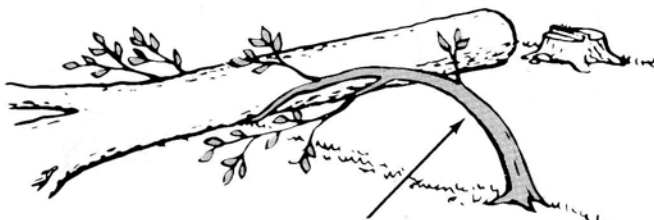
THIS IS A SPRINGPOLE BENT DOWN UNDER HIGH STRESS
