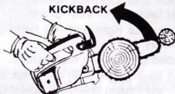
NOSE STRIKING ANY SOLID OBJECT (WILL CAUSE A KICKBACK)
