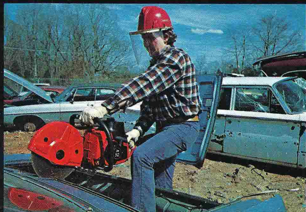
Cuts usable parts from wrecked cars for salvage.
