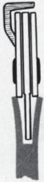
Fig. HC2— Chain will not run true in spread guide bar rails.
