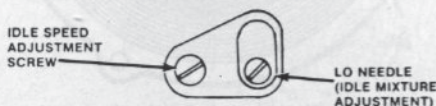
Fig. HL41-1—View showing location of idle mixture screw (I) and idle speed screw (S).
