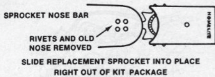
Fig. HC37—Install Power Tip® bar as outlined in text.
