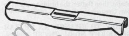
Fig. HC36—Use a depth gauge tool to accurately measure depth gauge height when filing.
