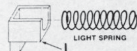
Fig. HL29-2—Note position of lug (L) when identifying high and low speed sliders. Be sure correct spring is installed in slider.
