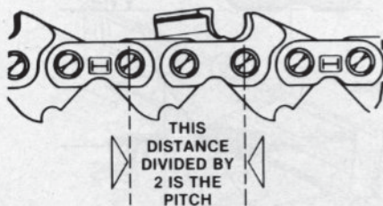
Fig. HC22—To determine chain pitch, measure distance between every other rivet as shown and divide by 2.
