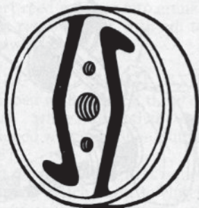
Fig. HL153—View of correct installation of clutch hub in drum.
