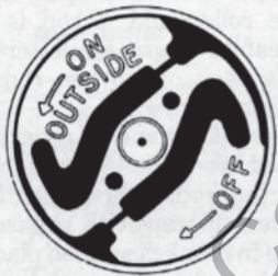
Fig. HL10A—View of correct installation of "S" type clutch hub in drum.
