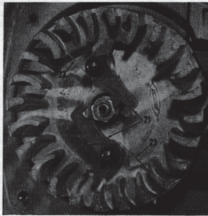
Fig. HL50A — When installing starter pawls (21), be sure that pawl return springs (23) are located in flywheel vanes so that they are parallel to the pawls as shown.
