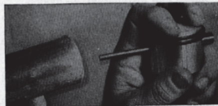
Fig. HL40—After removing snap rings, the piston pin can be tapped out using a 3/16-inch rod as shown or, on pistons with Spirol pin at exhaust side, by driving piston pin out with slotted driver (Homelite tool No. 23949).
