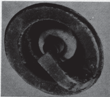
Fig. S3—Two stroke engine plug of correct heat range. Insulators light tan to gray with few deposits. Electrodes not burned.
