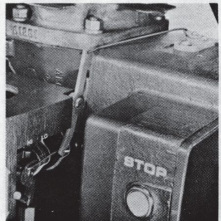
Fig. HL23—View showing proper installation of governor bellcrank and links. Generator engine not equipped with throttle (idle control) rod is shown.
