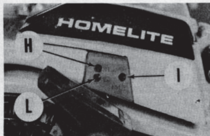
Fig. HL250—View of carburetor idle speed screw (I), high speed mixture screw (H) and idle mixture screw (L).
