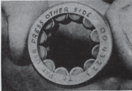
Fig. HL97—Roller type main bearing used at fly-wheel end of crankshaft is marked on one side, "PRESS OTHER SIDE". Be sure to observe this precaution when installing bearing in crankcase.
