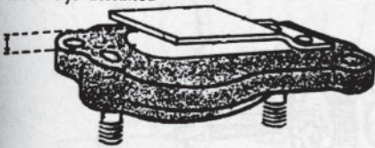
Fig. HL220—Reed lift distance should be 0.085 for model ZIP and 0.190 for WIZ and WIZ 55 with flat reed.
