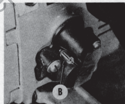
Fig. HL252—A neon bulb may be used to determine if ignition system is operating correctly. See text.
