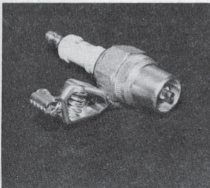
Fig. S2A—View of test plug which may be used for ignition troubleshooting.
