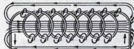
Fig. CS12—When a wire carrying an electrical current is wound in the shape of a coil or helix, the magnetic field surrounding loops of the wire tend to converge into a single electro-magnetic field as shown. If the loops of the coil are wound closely together, there is very little tendency for the electro-magnetic field to surround individual loops of the coil.
