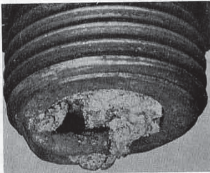
Fig. CS43 — Gray, metallic aluminum deposits on plug. (Seldom encountered). Piston damage due to pre-ignition. Overhaul motor and determine cause of pre-ignition.
