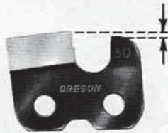
Check depth gauges every 3rd sharpening.
