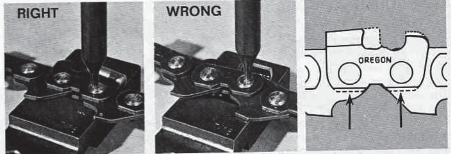
1. Fit chain into smallest slot of Chain Breaker so cutter is on top. Punch out rivets of damaged part.
