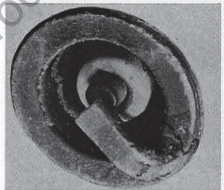
Fig. CS40 — Two cycle engine plug of correct heat range. Insulators light tan to grey with few deposits. Electrodes not burned.
