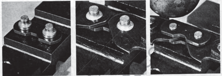
5. Dimple on tie strap faces out. Form rivet head with hammer.
