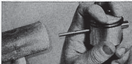
Fig. HL39 — After removing snap rings, the piston pin can be tapped out using a 3/16-inch rod as shown or, on pistons with Spirol pin at exhaust side, by driving piston pin out with slotted driver (Homelite tool No. 23949).
