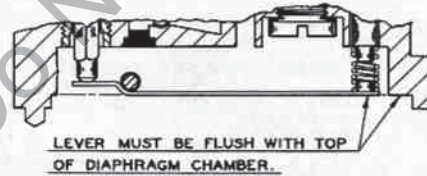
Fig. HL236—Cross-sectional view showing proper setting of fuel diaphragm lever (25—Fig. HL235).
