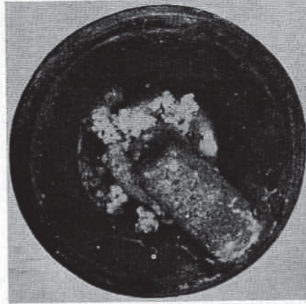
Fig. CS44 — Core bridging from center electrode to shell. Fused deposits sometimes have the appearance of tiny beads or glasslike bubbles. Caused by excessive combustion chamber deposits which in turn could be the result of; excessive carbon from prolonged usage; use of improper oil or incorrect fuel-oil ratio.
