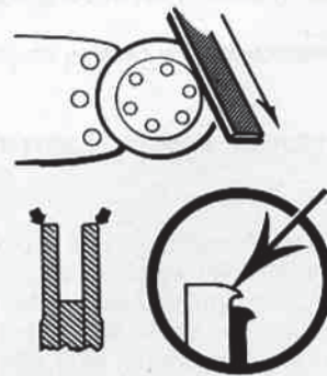
Fig. 33—Removing burrs from roller side plates.
