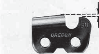
Check depth gauges every 3rd or 4th sharpening.
