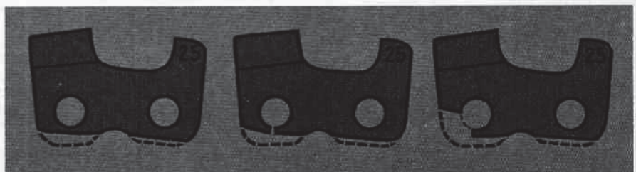
Fig. 38 —Cutting frozen wood causes cutters to wear, crack and break at the back rivet hole unless proper precautions are taken.
