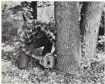
ENGINE TYPE — HOMELITE two cycle, loop scavenged single cylinder
