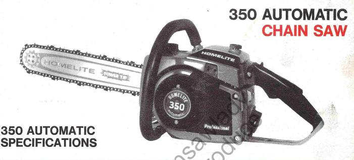
Type: Homelite 2-cycle, single cylinder, air cooled, loop scavenged, made of light alloys. Hemi-Head cylinder and full flow ram intake porting give greater efficiency and more power. Precision, chrome plated cylinder and steel rings for longer life.
