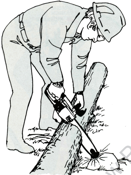
DEVICE RESTED AGAINST AN OBSTRUCTION TO PREVENT CHAIN DAMAGE
