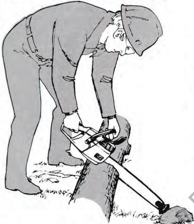
DEVICE RESTED AGAINST AN OBSTRUCTION TO PREVENT CHAIN DAMAGE
