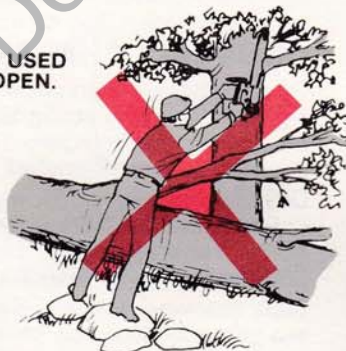
OPERATOR HAS POOR CONTROL OF SAW IF HE OVERREACHES OR CUTS ABOVE CHEST HEIGHT.
