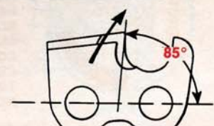
2. SIDE PLATE ANGLE OF 85° TO LINE OF CHAIN TRAVEL. MAY BE 85° TO 90° AS LONG AS ALL CUTTERS HAVE THE SAME ANGLE.
